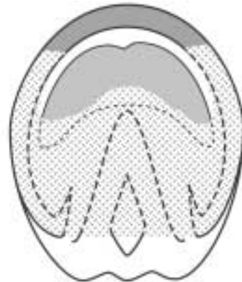
Fig 2: A schematic diagram showing the optimal area of the ground surface of the foot that can be recruited to bear weight (hatched area) without applying pressure to the dorsal margin of the distal phalanx or the adjacent wall.
