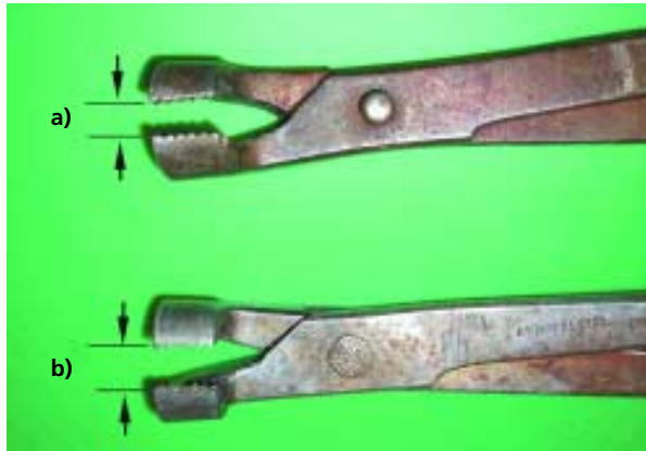
Fig 6: The width between the jaws is wider for maxillary cheek tooth extractors (b) than for those used for extracting mandibular teeth (a), and there is variation in the width of the teeth between individual horses.
