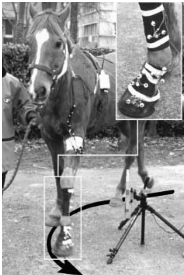
Fig 1: Photograph of the experimental setup. Arrow indicates the movement of the horse in a left turn, on a path that was drawn on the ground. Zoom box shows triads of markers affixed to the tip of the intracortical pins.
